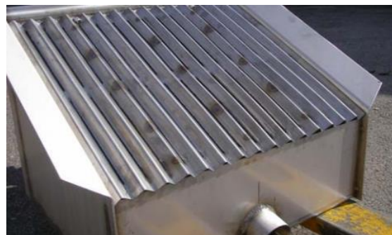
Illustration 6-10 Rack bar of a Tyrolean weir (HZI, n. y.)
