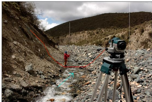
Illustration 12-3 Cross sections of the Arroyo Morteritos, 1) At the planned weir, above the Parshall flume Tracer Input, 2) Tracer input behind the Parshall flume, tracer mediation behind th çe Parshal flume
